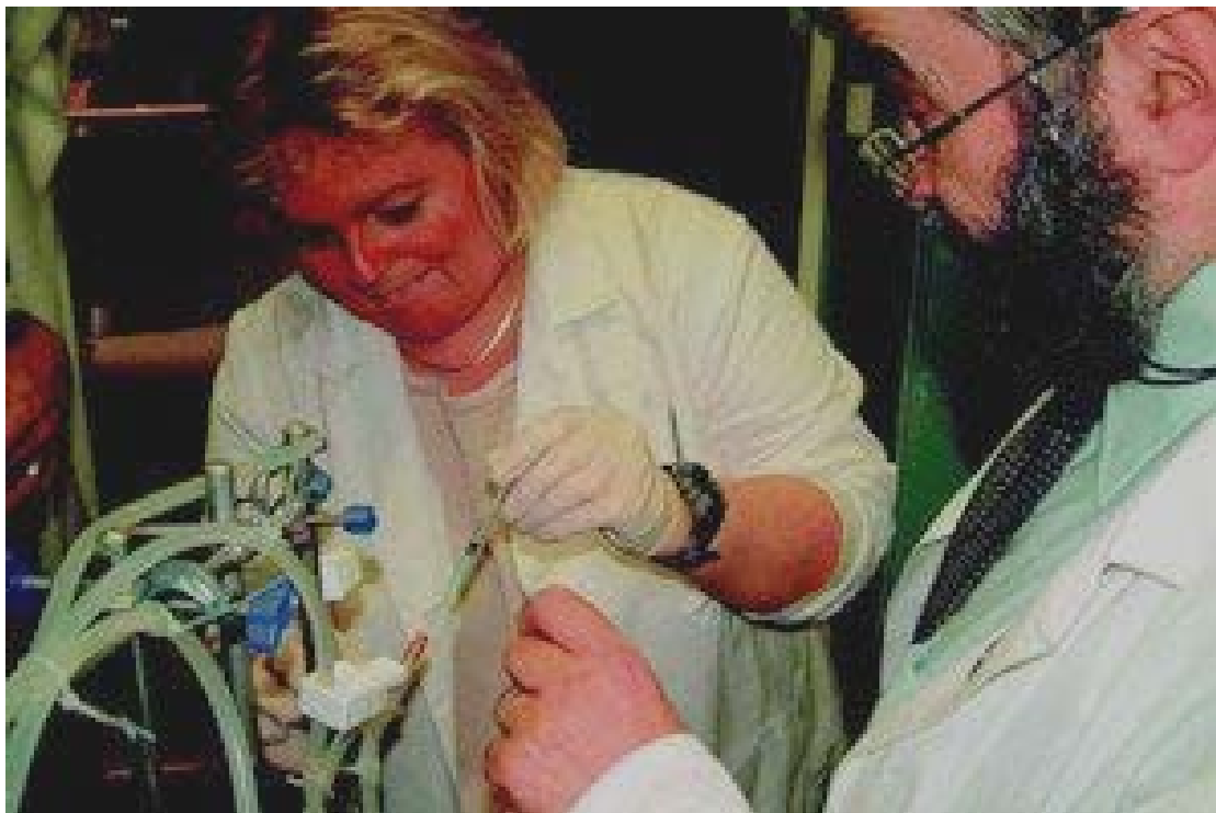
Soil columns being injected with Tc tracer at Manchester Royal Infirmary. (Credit: Image courtesy of University of Manchester)
